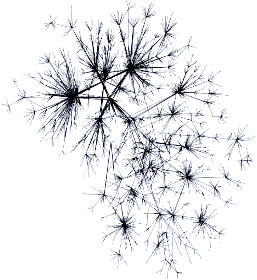
Figure 13.1: Most companies have an official list of the networks in their intranet. This list is almost always incomplete. In this especially well-run network, only a couple of links, shown in bold, were unknown.
